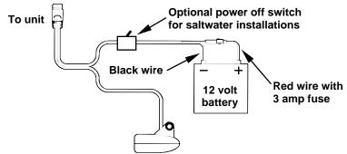
Power and transducer connections for the X37TX and X47TX sonar units (direct battery connection shown).
